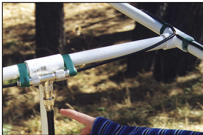
A close-up of the antenna feedpoint. On the element to the right, you can also see the 25-Ω feedpoint arrangement that is detailed in Figure 4 .
